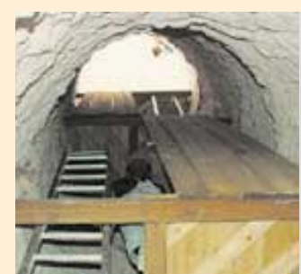
Trial shaft to assess reserves at Al Jalamid
